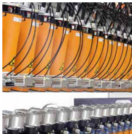
Figure 18: Industrial delamination detection on wood-based materials with air-coupled ultrasound. Multiple transmitter/receiver channels are distributed across the width of a panel to ensure complete monitoring during ongoing production.
