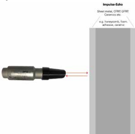
Figure 2: ACUT with the Impulse-Echo Method
